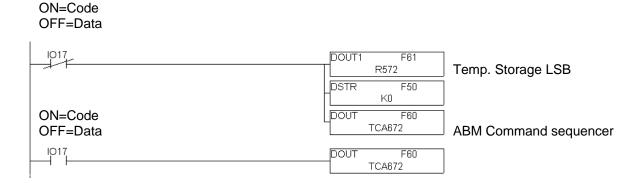
Command used when transferring 16 bit data.
