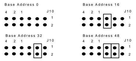
A read or write to a slot within a Bridge CPU's address range will cause the "ADDR" LED to flash. Module address = Base Address + Slot Number x 2.
