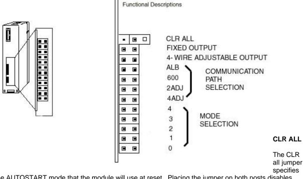
the AUTOSTART mode that the module will use at reset. Placing the jumper on both posts disables AUTOSTART and waits for a space bar character in port 1. Placing the jumper on one post allows the module to use the last stored AUTOSTART parameters (this is the default factory setting).
