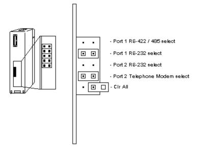
The communication interface type for port 1 is selected by placing a jumper on one of the port 1 options, either RS422/485 or
