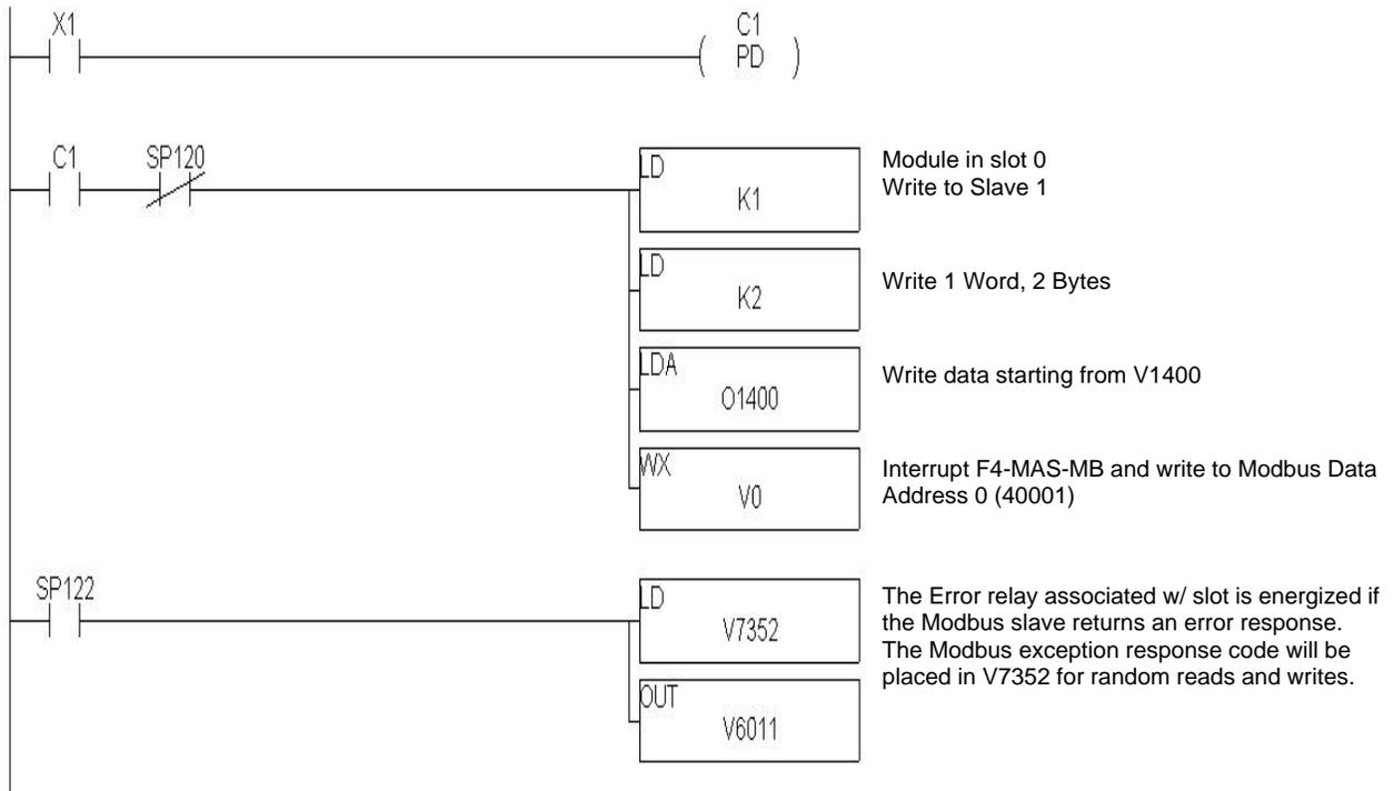
LD     Kssaa - ss is the slot number where the F4-MAS-MB is located.
