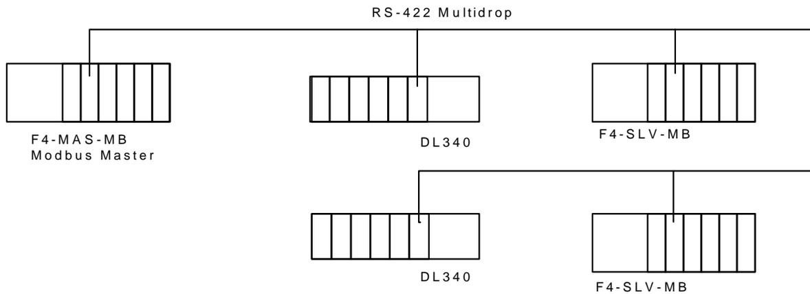
**Example 2** - F4-MAS-MB as Modbus Master with DL340's (Need FA-ISONET converter for each 340) and F4-SLV-MB's as Modbus Slaves. Computer connected to the DL340 or DL440 Slave port (using DirectNET protocol) monitoring all slave data.
