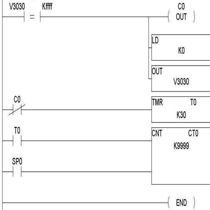
When V3030 is equal to zero turn ON C0 and set V3030 = 0
