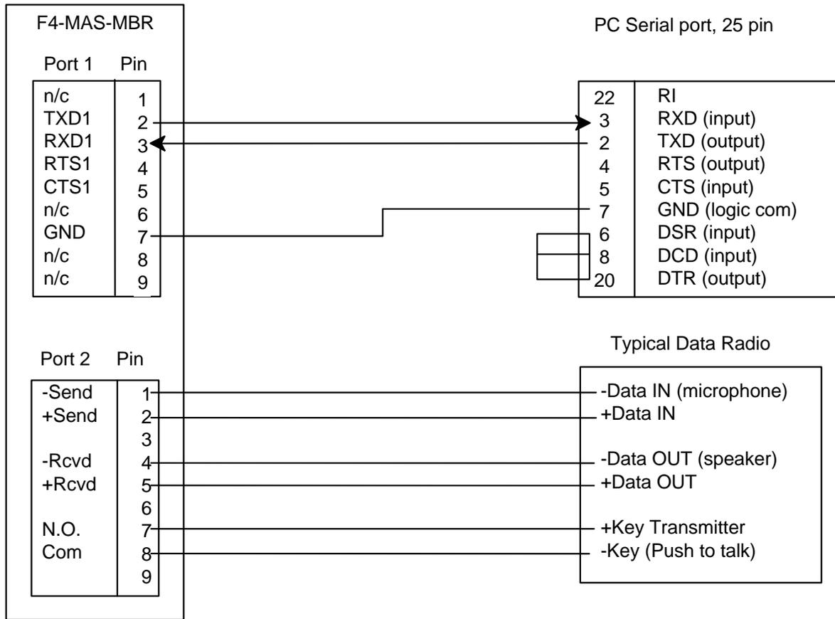
\* For half duplex (2-wire) operation, connect Port 2 pins 1 to 4 and pins 2 to 5.
