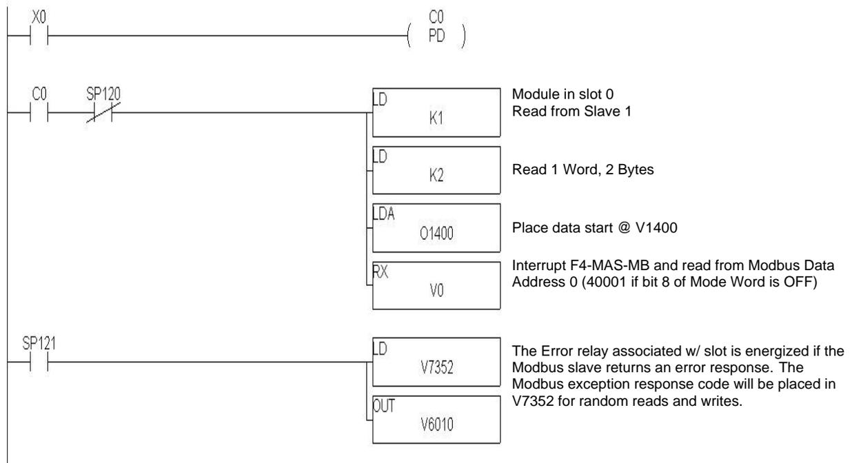
LD     Kssaa - ss is the slot number where the F4-MAS-MB is located
