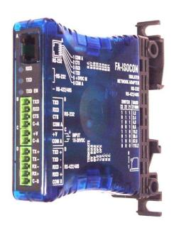
The FA-ISOCON Universal Isolated Network Adapter is used to place *Automationdirect* CPUs and other RS-232 devices such as operator interfaces and industrial computers on a RS-422 (4-Wire) or RS-485 (2-Wire) multi-drop network. The Network Adapter converts RS-232 signal levels to isolated RS-422 or RS-485 signal levels. All *Automationdirect* CPU ports that support multi-drop networking protocols can be used with the FA-ISOCON.
