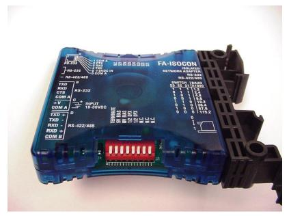
The dipswitches are located under a switch cover. Remove the switch cover by pressing down on the plastic ridges and sliding the switch cover out.
