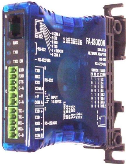
The FA-ISOCON Universal Isolated Network Adapter is used to place **Automationdirect** CPUs and other RS-232 devices such as operator interfaces and industrial computers on a RS-422 (4-Wire) or RS-485 (2-Wire) multi-drop network. The Network Adapter converts RS-232 signal levels to isolated RS-422 or RS-485 signal levels. All **Automationdirect** CPU ports that support multi-drop networking protocols can be used with the FA-ISOCON.
